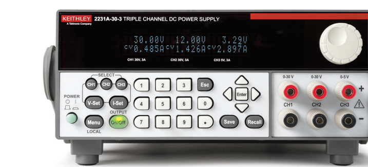
Low-Voltage DC Supply - Powers Gate Drive Electronics
