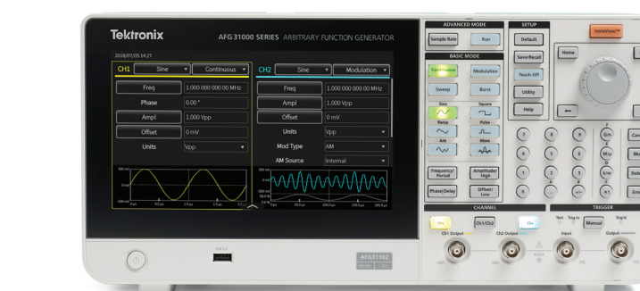
Signal Source - Provides Gate Drive Signal
