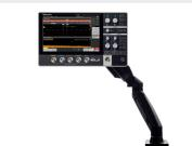
Built in VESA interface enables use of off-the-shelf VESA accessories. Optional rack mount, protective case, and kickstand enable different uses.
